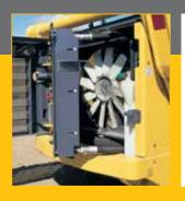
A new swing-open rear door, swing-up engine cover, and swing-out cooling package provide quick and complete access to the engine compartment.
