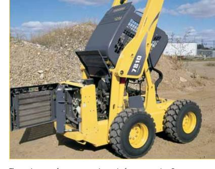
The engine cover features gas-spring assist for easy opening. Removable side panels provide quick access to service points and filters. A build-in hydraulic pump lifts the entire ROPS/FOPS structure up and out of the way for complete access to traction drive and hydraulic components. An optional electric pump is also available for ROPS lift.
