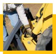
GEHL All-Tach<sup>TM</sup> system is compatible with most skid loader attachments and makes connecting as well as disconnecting fast and easy.
