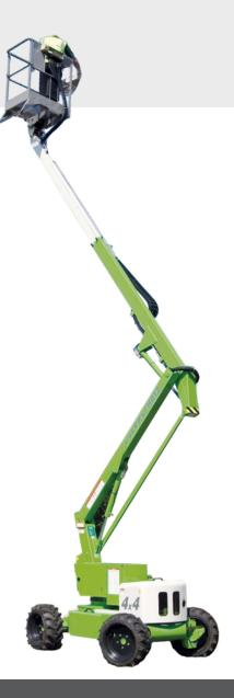
With its compact dimensions and class-leading working envelope, the Height Rider 12 has always been versatile and reliable. Add to this a low weight chassis and a powerful 4-Wheel-Drive system and you've got the Height Rider 12 4x4 (HR12 4x4) - one of the most complete 12m (40ft) self propelled boom lifts available.
